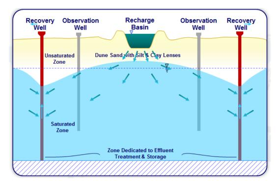
Figure 20 Soil Aquifer Treatment at Shafdan<sup>978</sup>
