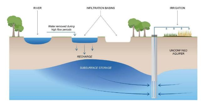
Figure 8 Conceptual representation of a managed aquifer recharge system showing capture of flood flow, recharge/reinjection and recovery for irrigation 688
